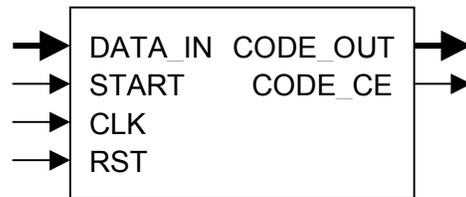
Figure 2. Schematic symbol of the decoder
