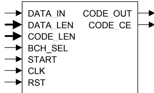
Figure 2. Schematic symbol of the decoder
