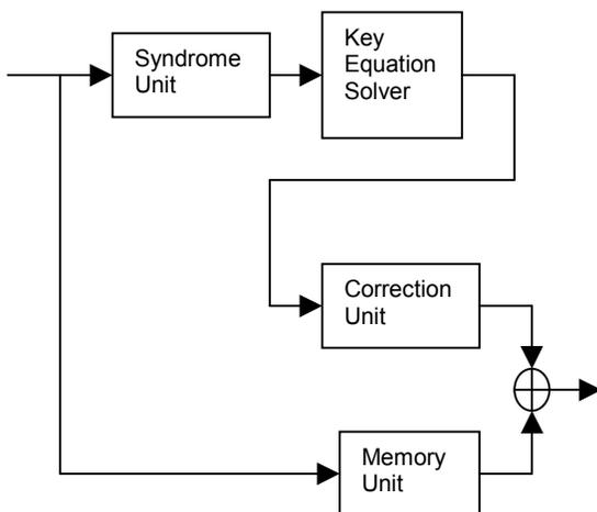
Figure 1. Block diagram of the BCH decoder.
