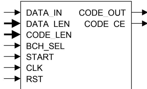
Figure 2. Schematic symbol of the encoder
