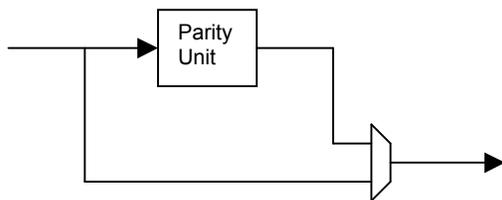
Figure 1. Block diagram of the BCH encoder.
