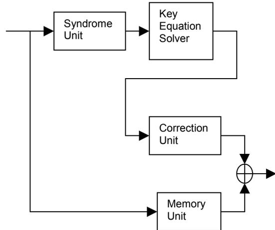
Figure 1. Block diagram of the Reed-Solomon decoder.
