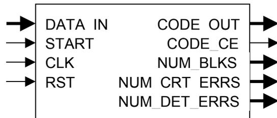
Figure 2. Schematic symbol of the decoder
